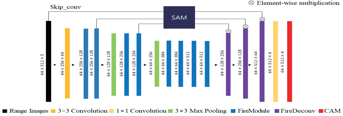
Fig. 2. An architecture of the proposed network. Each convolution layer is followed by ReLU activation. (Best viewed in color)
