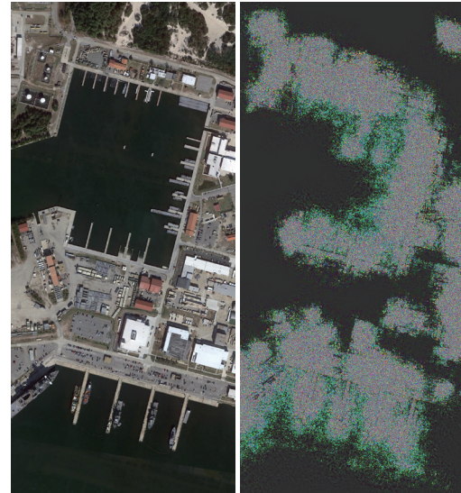
(a) Input image (b) Epsilon lrp result Fig. 1. Example of applying epsilon lrp model explanation to the satellite image input and object detection model
